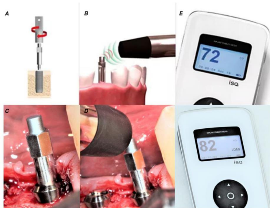
Figure I.25 The resonance frequency analysis (RFA) [56]: (A) insertion of the measurement adapter, (b) resonance frequencies measured with the device, (c) implant with adapter in situ, (D) RFA-measurement from the vestibular side, and (E) implant stability meter with implant stability quotient (ISQ) values for the evaluation
