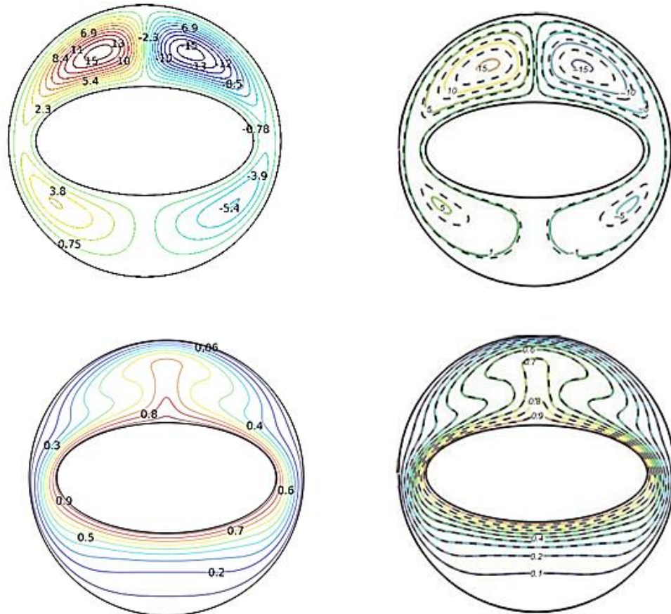
Figure 27 Streamlines (top) and isotherm contours (bottom) of the current study [right] and Sheikholeslami et al.[6] [left].
