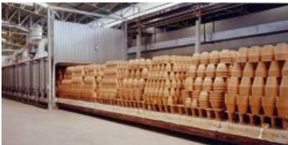
Figure 1.12: four à Wagonnets
