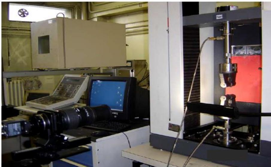
**Figure II.14** Machine de traction (Lloyd LR/10KN).
