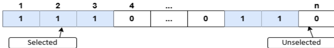
Figure 3.1: Representation of BDE for FS solution.
