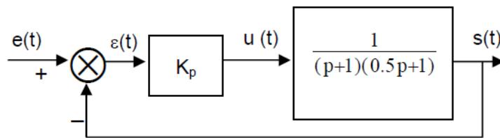
Figure 2.5: Proportional controller in control process
