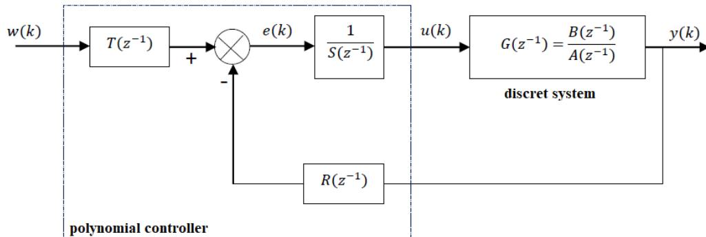
Figure 4.1: polynomial control schema
