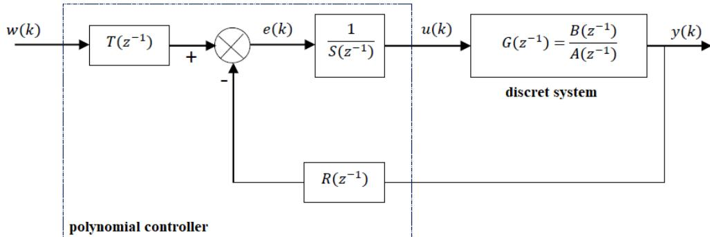
Figure 4.1: polynomial control schema
