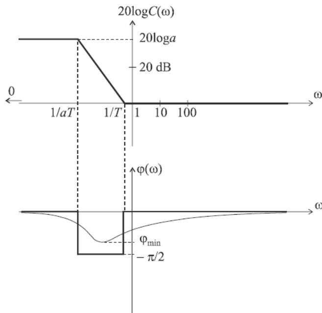
Figure 2.11: Bode plot of a phase delay corrector
