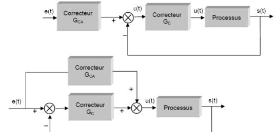
Other configurations, such as **feedforward correction**, are also widely used depending on the system's requirements.
