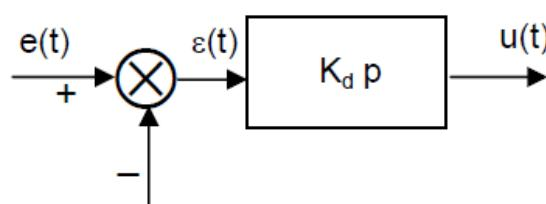
Figure 2.8: Pure Derivative Action Correction
