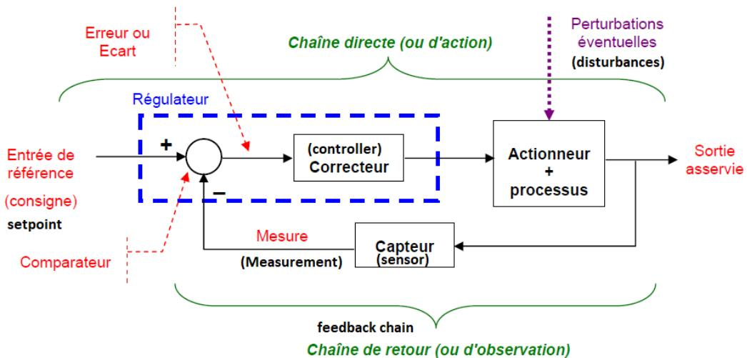
Figure 1.2: Detailed control loop
