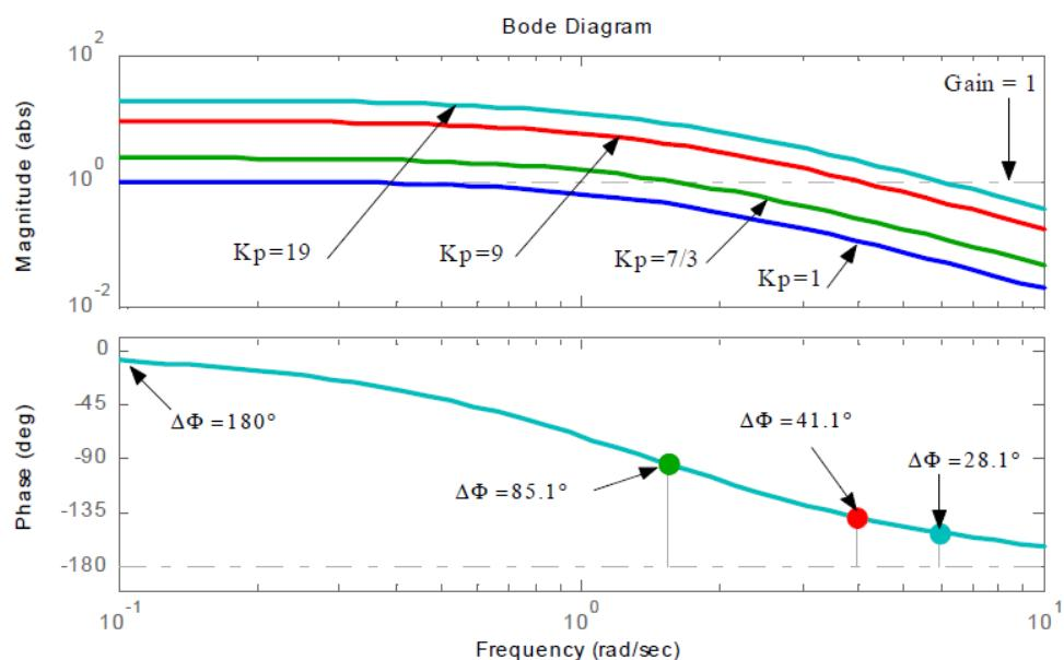
Figure 2.7: Effect of the proportional controller on stability margins
