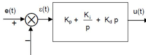
Figure 2.9: Proportional, integral and derivative (PID) correction
