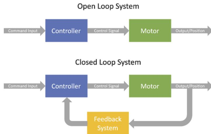
Figure 1.3: open loop Vs closed loop
