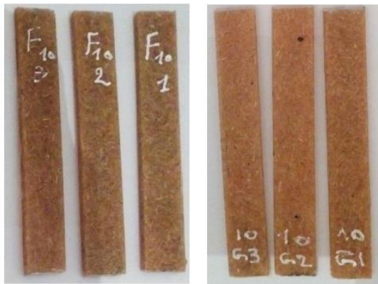
Fig. 2. Polyester/Alfa composite specimens for bending test.
