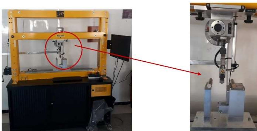
Figure II.16: Bend testing machine.
