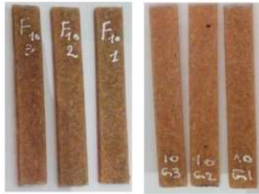
Figure II.12: polyester/alfa composite specimens for bending test.
