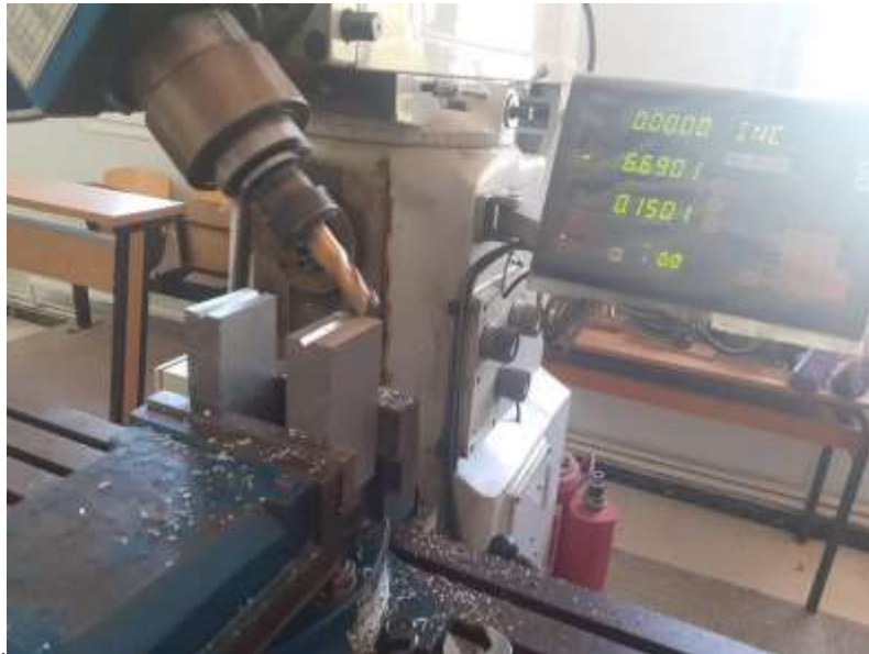
Figure II.15 : Manufacturing of Test Supports : Milling Operation with Digital Control.
