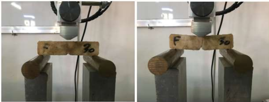
Figure II.19: Composite specimens SENB during three-point bending test.
