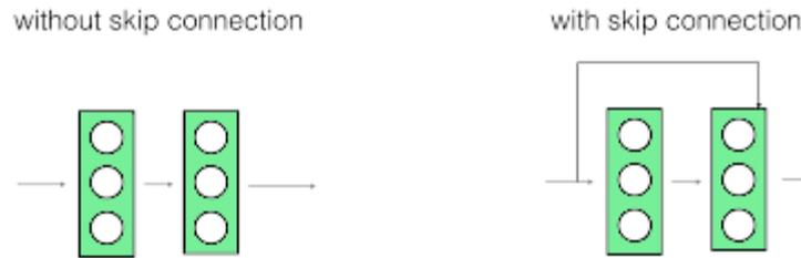
**Figure 4.19:** Concept of Residual blocks in ResNet networks.
