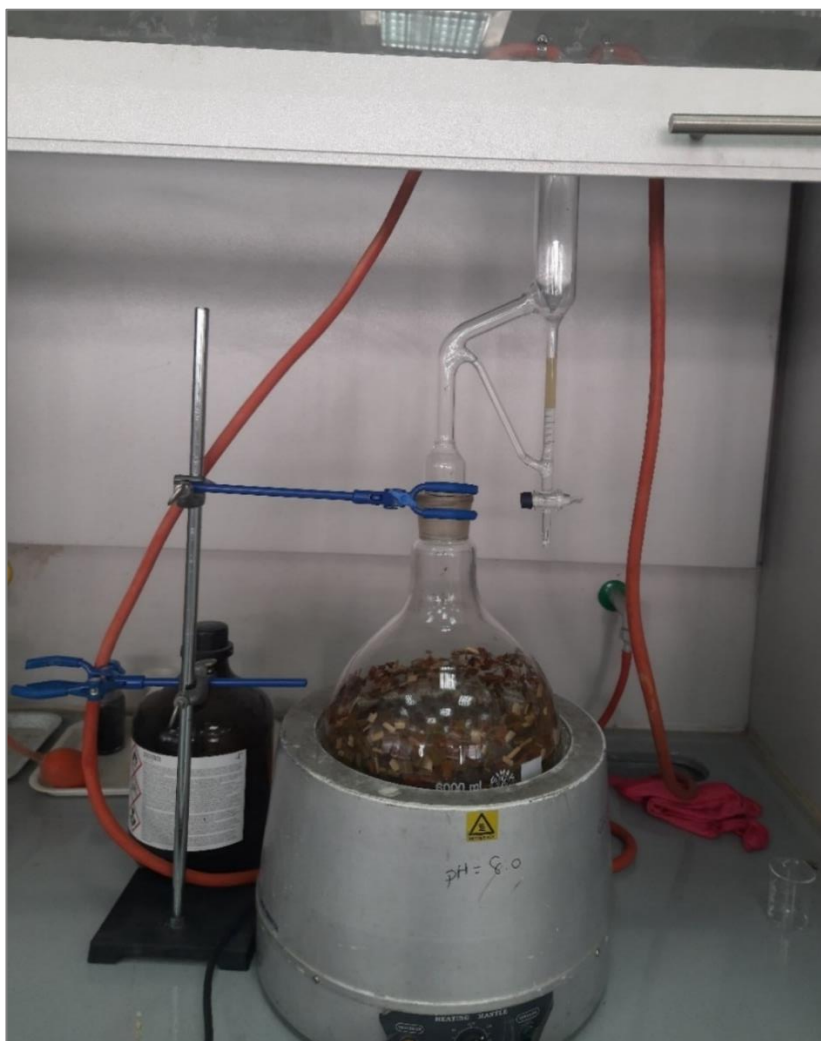
Figure 41: Essential oil extraction through hydrodistillation using a Clevenger-type apparatus
