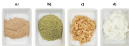
**Figure 2.** Raw fibers of DP (a), raw fibers of FP (b), delignified fibers (c) and bleached fibers (d)
