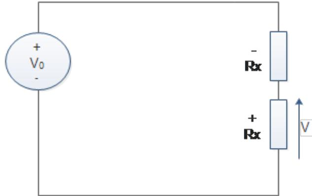
**Figure 3.5:** Measurement of a resistance  $R_x$  using the Push-Pull circuit
