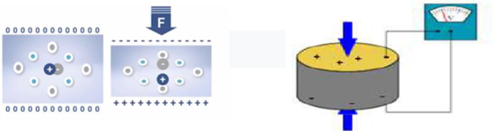
**Figure 1.9:** Piezoelectricity
