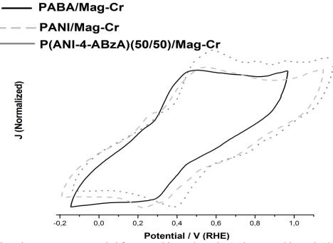
**Figure. 4:** Cyclic voltammograms recorded for a graphite carbon electrode covered by poly(4-ABzA)/Mag-Cr, polyANI/Mag-Cr and copolymers poly(ANI-4-ABzA)(50/50)/Mag-Cr in 1M HClO<sub>4</sub> solution. Scan rate 50 mV s<sup>-1</sup>.
