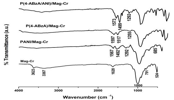
**Figure. 2:** FT-IR adsorption spectra of the Cromium-Montmorillonite (Mag-Cr) poly(4-ABzA-co-ANI)/Mag-Cr, poly(4-ABzA)/Mag-Cr and polyANI/Mag-Cr nanocomposites.
