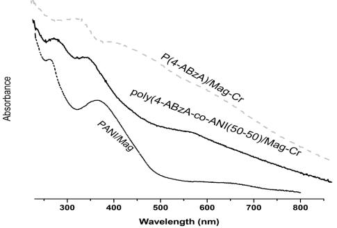
**Figure. 3:** UV-vis spectra of the : poly(4-ABzA-co-ANI (50/50))/Mag-Cr, poly(4-ABzA)/Mag-Cr and polyANI/Mag-Cr nanocomposites.
