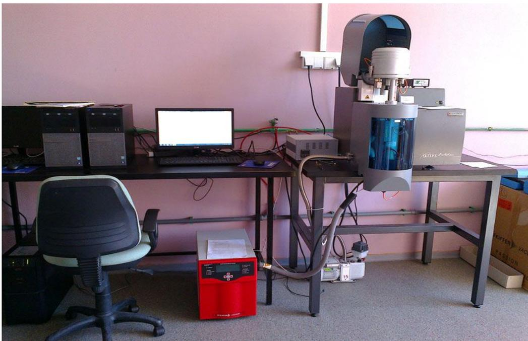
**Figure 12:** Appareil TG-Setaram Setsys Evolution 16
